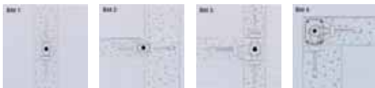
butt joint of two walls wall connection butt joint and wall connection wall and ceiling connection
