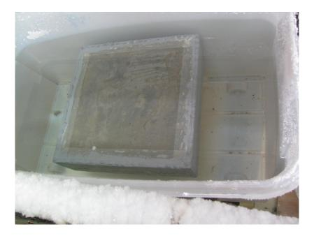
Test procedure: storage in the water tank at temperature of  $(21\pm2)^{\circ}$ C. Thaw stage.
